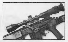
Nimrod 6X40mm scope attached to Galil Sniper Rifle with a quick-release side-rail mount features an excellent Dragunov/RPG-7-type reticle range finder.
